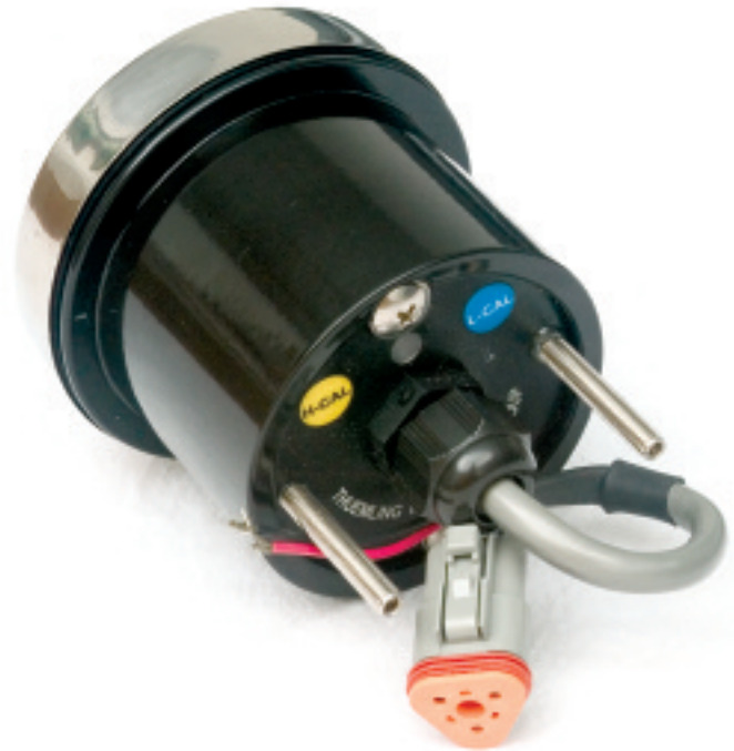
▲ 'EG' SERIES GAUGE - REAR DETAIL
