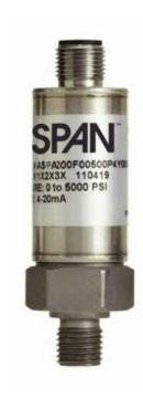
**Environmental Data** Temperature -40 to 125°C (-40 to 250°F) Operating Storage -40 to 125°C (-40 to 250°F) Thermal Limits Compensated Range 0 to 55°C (32 to 131°F) TC Zero <± 1.0% FS TC Span <± 1.0% FS Other Shock 100G, 11 msec, 1/2 sine 20G peak, 20 to 2400 Hz. Vibration EMI/RFI Protection: Yes Rating: IP-66 (optional IP-67)
